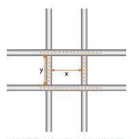
SPECIFIED MESH BI-AXIAL WELDED
